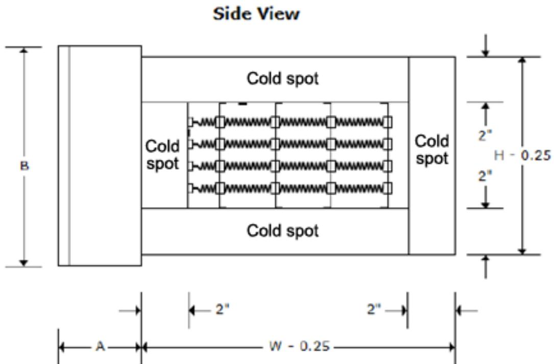
These cold spots can be used on all four sides of the heater (box, end, top, bottom) based on what is required, but it is highly important to make this request at the ordering stage. Modifications cannot be done to add cold spots once heaters are built.
