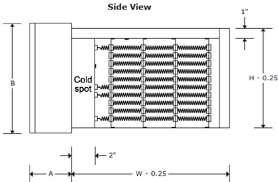
Another situation where cold spots can be used is in installations where the air velocity is lower than the minimum velocity required for the PID switch (300 FPM) or Electronic Airflow Sensors (EAS) (100 FPM). In this situation, cold spots are a good solution, which can reduce the area through which the airstream passes and increase the velocity to make the PID and EAS while making sure the thermal cutouts and coil are fully exposed.
